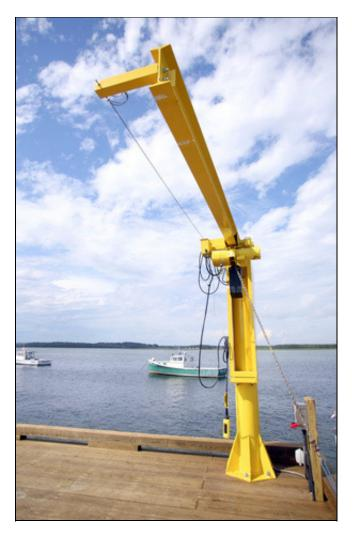
The new municipal pier at Pine Point in Scarborough has two hydraulic hoists that can help load gear and bait directly from trucks to boats, saving time and effort.
